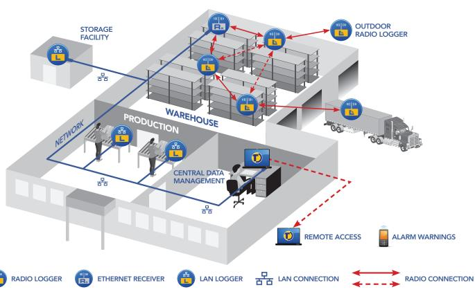
Tinytag Connect is designed for flexibility and ease of use: Radio and LAN data loggers can be mixed and matched within an application to meet particular site layout and infrastructure requirements. Monitoring parameters including temperature, RH, low voltage, current and count inputs; and a choice of indoor or outdoor radio units.
